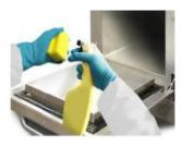
6. Spray Merrychef cleaner onto a sponge and wipe over the cavity and door, avoiding the door seal and internal top plate.
